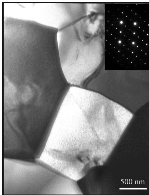
Fig. 4. Bright field TEM image of BMT sample sintered at 1580 °C for 20 h. The insert shows the SAD pattern from a single 1:2 ordered domain.
